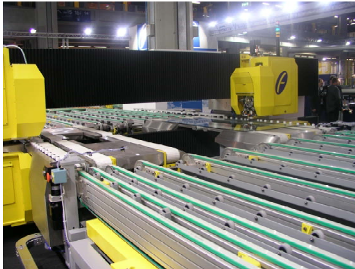
main entry conveyor
